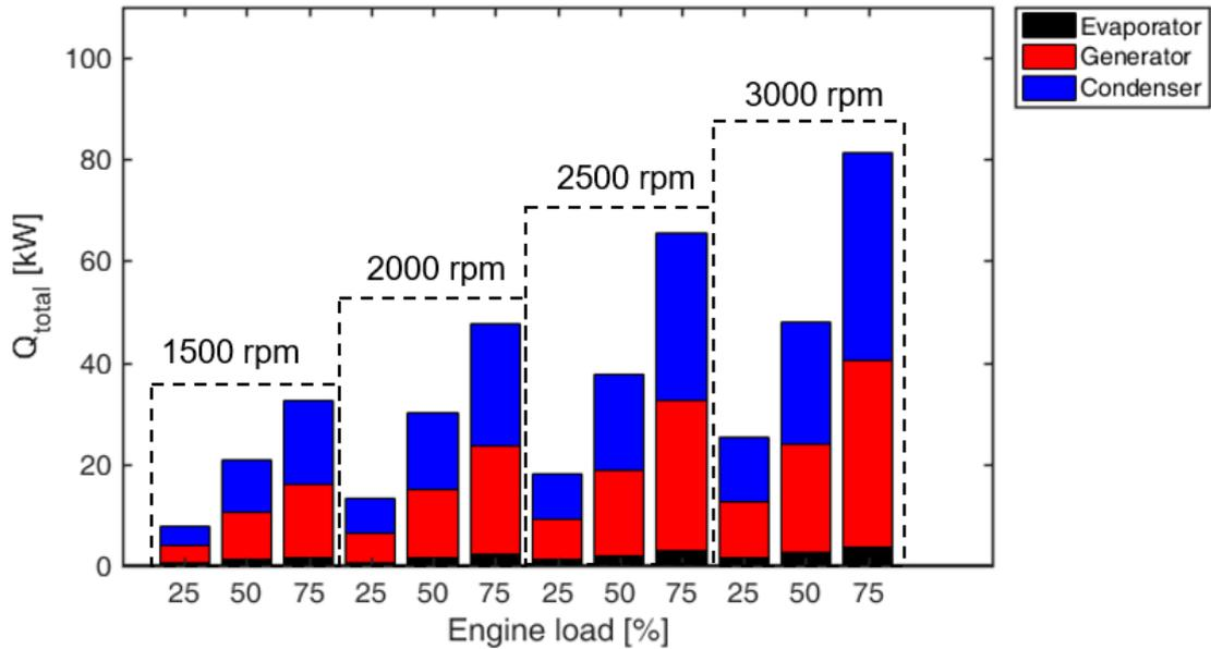
Figure 8. Condenser, generator and evaporator heat exchanged over different engine operating points in *design* study
