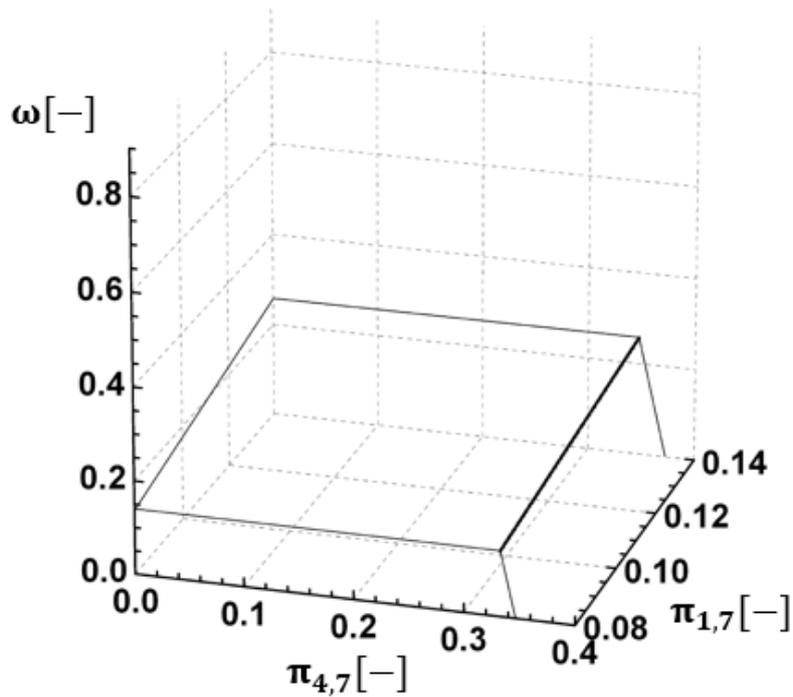
Figure 4. Ejector map optimized for  $P_7 = 40 \text{ bar}$ ,  $P_4 = 13 \text{ bar}$ ,  $P_1 = 4 \text{ bar}$ . Optimum dimensions correspond to  $d_{n,o} = 2.8 \text{ mm}$ ;  $d_m = 3.5 \text{ mm}$
