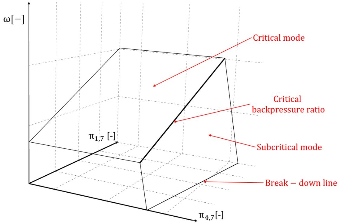
Figure 3. Ejector characteristic surfaces
