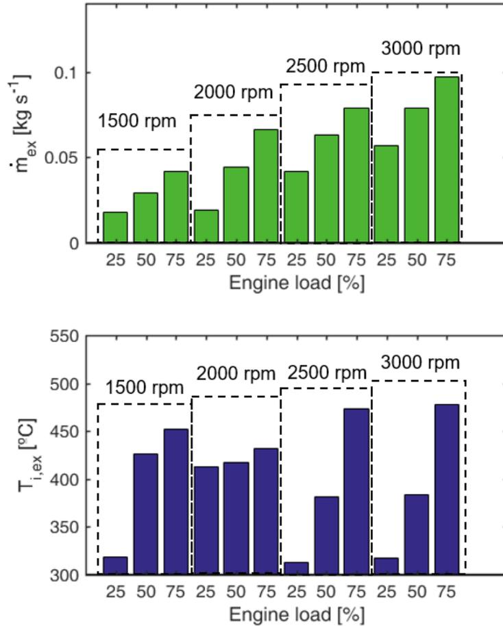
Figure 5. Exhaust temperature and mass flow over different engine operating points
