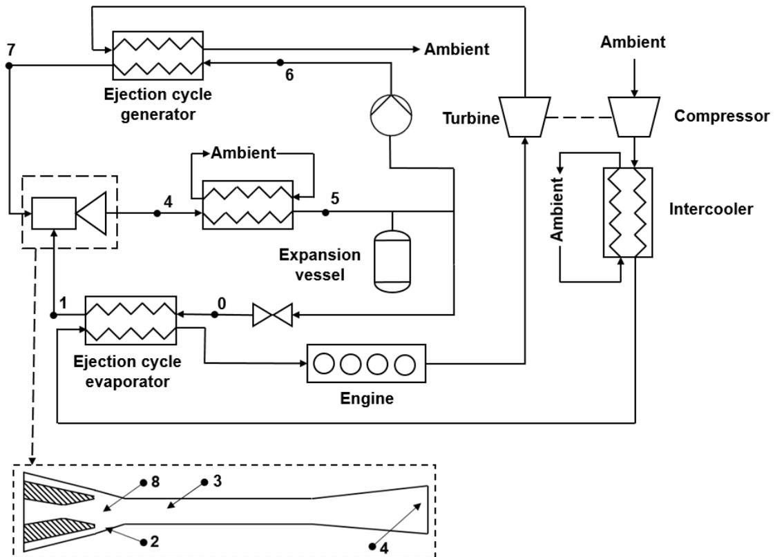
Figure 1. Ejection cycle arrangement intended to cool down engine intake
