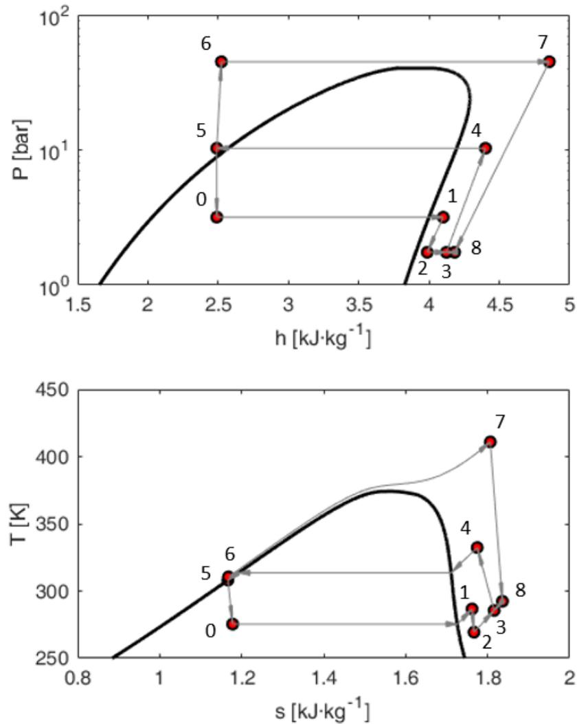
Figure 2. P-h and T-s diagrams of ejection cycle under investigation (R134a)
