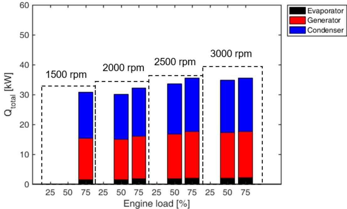
Figure 10. Condenser, generator and evaporator heat exchanged over different engine operating points in *off-design* study
