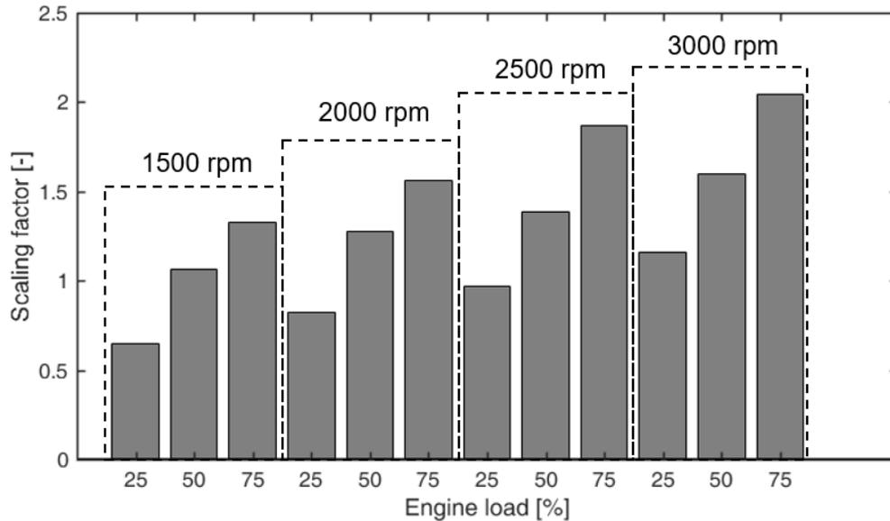
Figure 9. Required ejector scaling factor over different engine operating points
