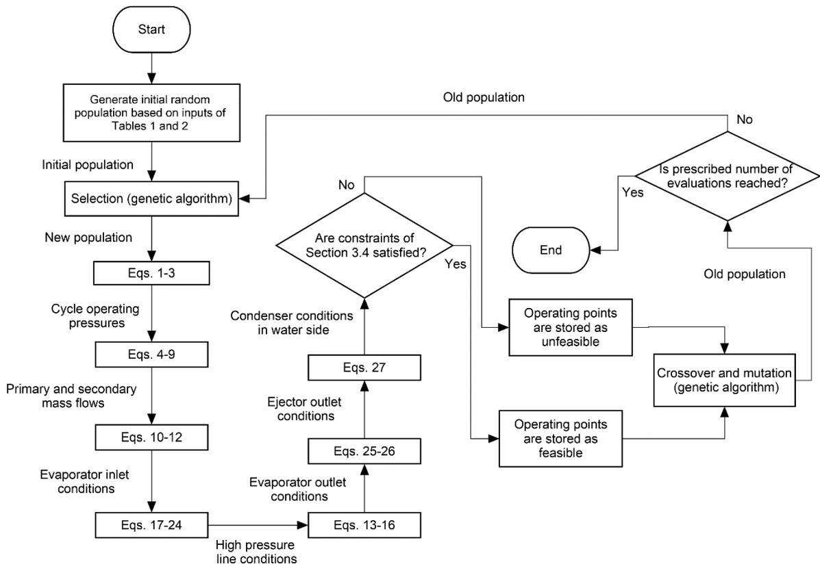
Figure 6. Flow diagram of the solving procedure
