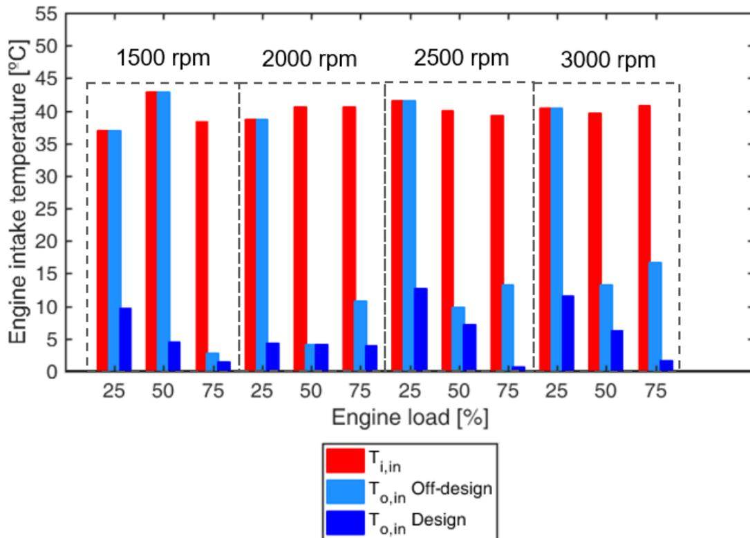
Figure 7. Engine intake temperature after cooling effect of ejection cycle in both *design* and *off-design* conditions
