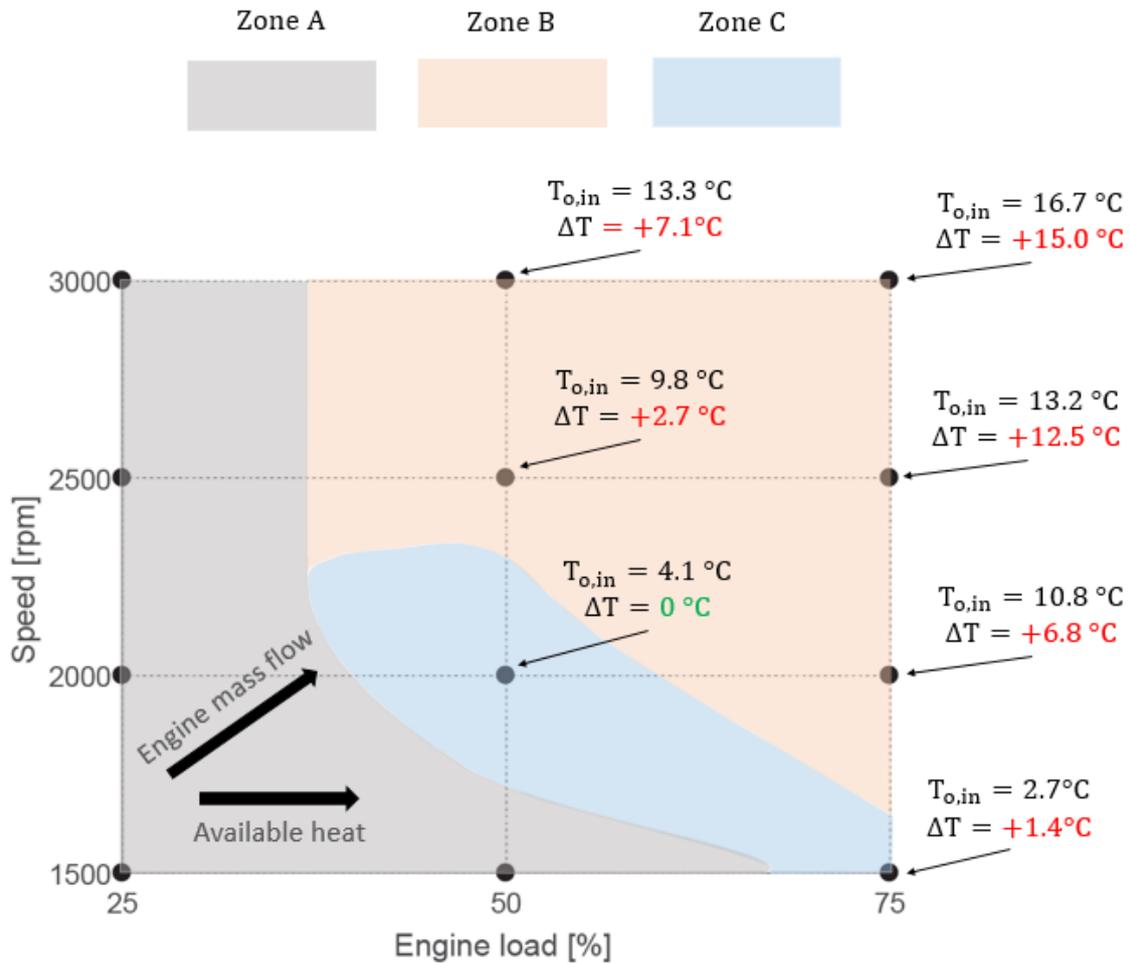
Figure 11. Ejection cycle performance degradation over different engine operating points
