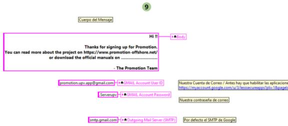
(a) Componentes del "block diagram" registro (5/7)
