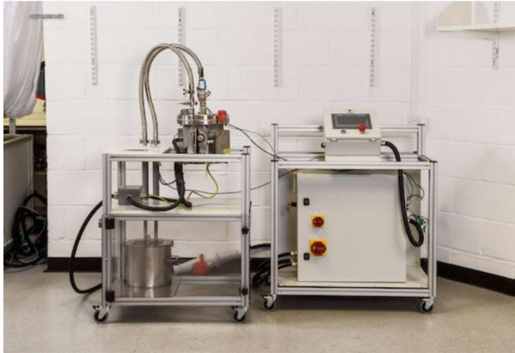
**FIGURA 4.** Calentador óhmico a escala laboratorio. ("The C-Joule Ohmic Heater Range by C-Tech Innovation", Model C-Joule LAB 150).
