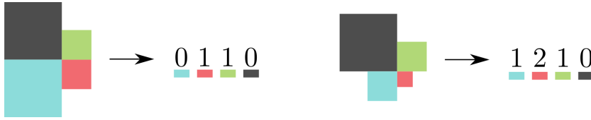
Fig. 3: 2D example of SPR patch coding. The patch on the left has code number 0110 and the patch on the right is number 1210.
