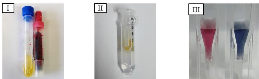
Figure S13. Images illustrating the procedure followed for measuring 5-HT in real human blood as described in the Experimental section. First, blood was centrifuged to separate serum (yellow phase) from red blood cells ( I ). Next, proteins were removed from serum using centrifugal filters giving a colorless solution ( II ). Finally, serum samples were mixed with the probe 1 and measured in the spectrophotometer ( III ).
