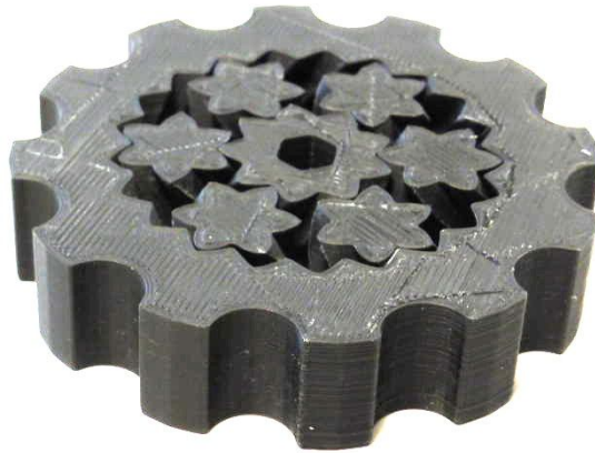
Figure 5. 3D printed gear.[14]
