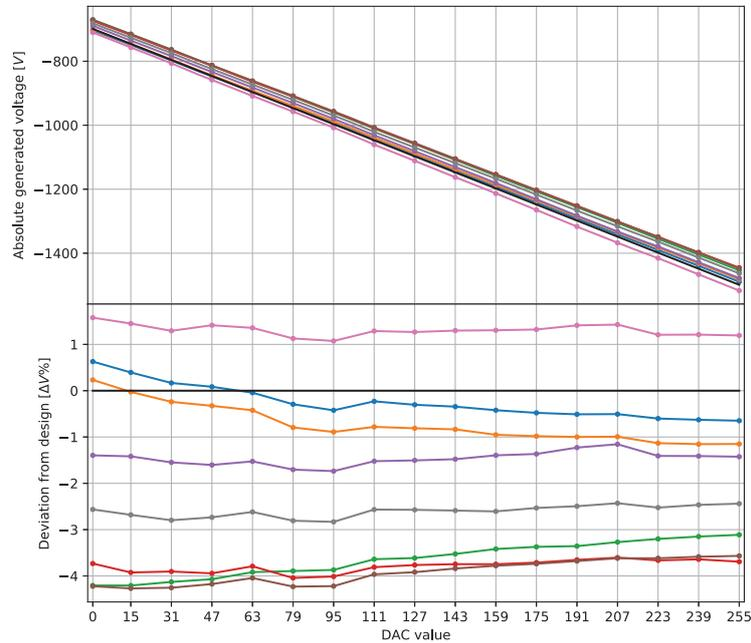
**Fig. 19** HV produced by a sample of PMT bases against a set PROMiS DAC value. The top plot shows the absolute voltage for eight selected bases, while bottom plot shows the relative deviation from the design voltage, where  $\Delta V\% = (V_{DAC} - V_{design}) / V_{DAC} \times 100$ . The black line represents the design value.
