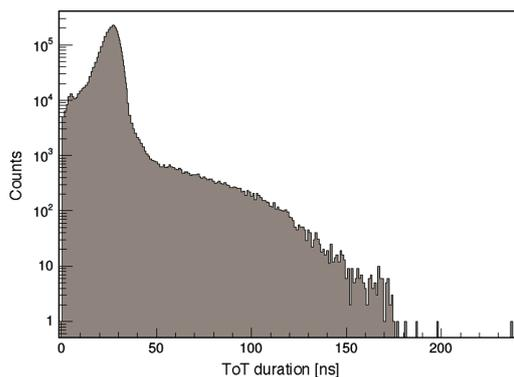
**Fig. 7** ToT distribution from one DOM of a deployed KM3NeT DU. All the channels have been calibrated in order to harmonize the ToT data arriving from different PMTs. The represented data correspond to both background and muons. The calibration process consists of tuning the HV until an spe provides a ToT between 26 and 27 ns. This ToT corresponds, on average, to a gain of  $3 \times 10^6$ .
