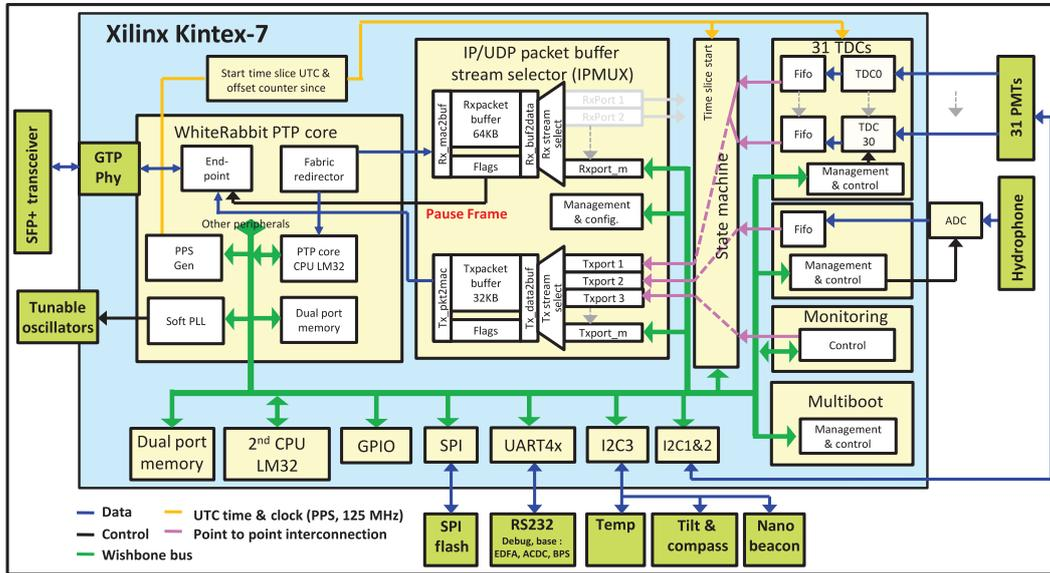
Fig. 5 Block diagram of the CLB FPGA firmware.
