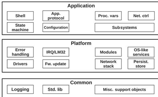
Fig. 10 Layers and modules of the CLB embedded software.
