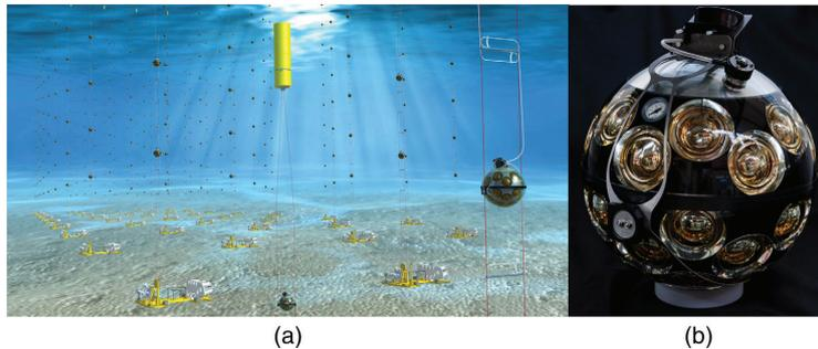
**Fig. 1** (a) Artistic illustration of the KM3NeT detector. Note that the illustration is not to scale and that sunlight will not actually reach the depths at which the KM3NeT detector is deployed. (b) A picture of the KM3NeT optical module with the fly's eye organization of the PMTs and the cap of the aluminum cooling "mushroom" visible. The titanium collar around the module supports the connection to the ropes of the DU.
