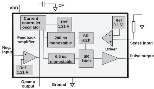
Fig. 18 Block diagram of the CoCo chip.
