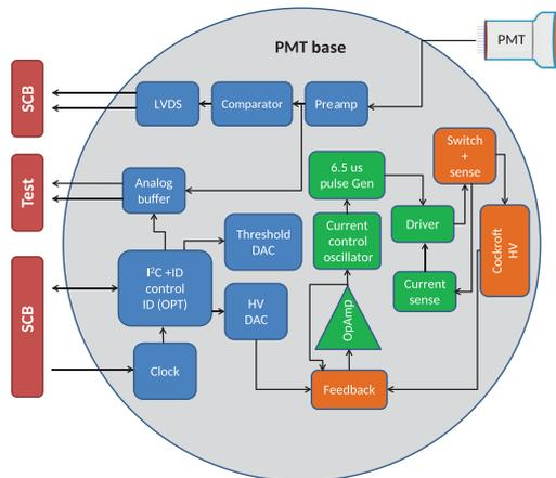
**Fig. 16** Block diagram of the PMT base. CoCo subsystems are represented in green, front-end mixed signal ASIC (PROMiS) subsystems are represented in blue, while discrete components are represented in orange.
