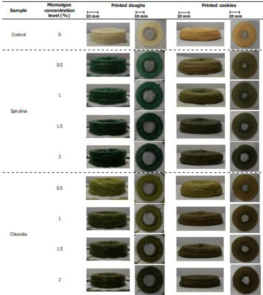
Figure 4. Example of 3D printed samples (layer height 1.3 mm and filament diameter 26 mm) before and after baking process.
