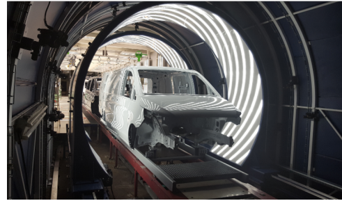
(b) QEyeTunnel system developed in Mercedes factories ( video [9]).
