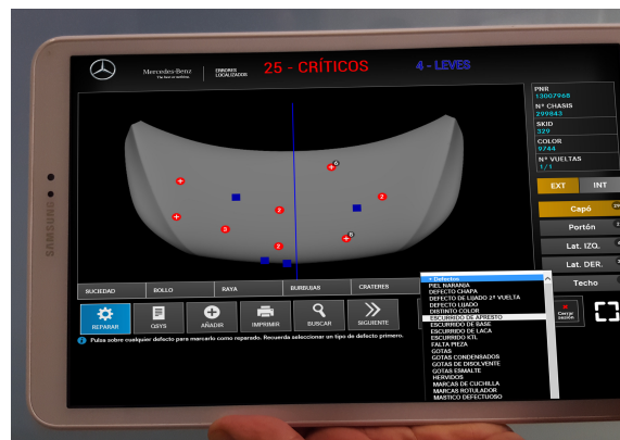
(c) QEyeTunnel worker interface PAD-based installed in Mercedes-Benz factory.
