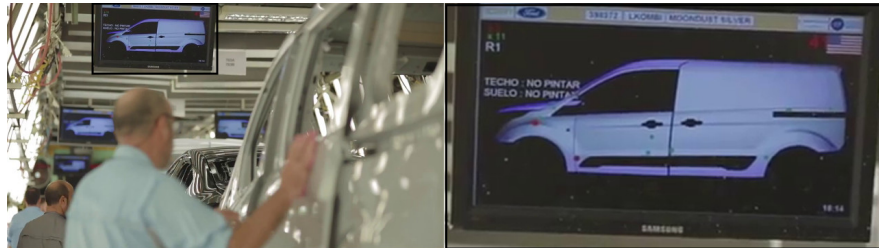
(a) AIS worker interface installed in Ford factories, see the following ( video [12]) for more details.
