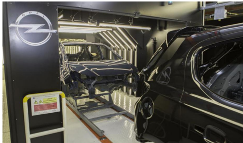
(c) 3DJ Vision system developed in Opel factories ( video [10]).
