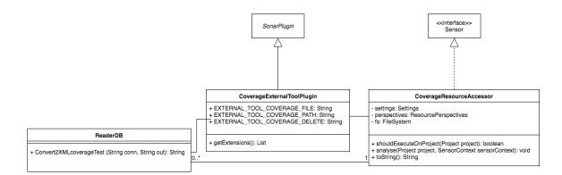
Figure 11: Class diagram of the coverage analysis module/plugin
