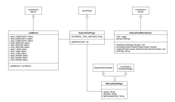
Figure 7: Class diagram of metric plugin for a specific external metrics tool
