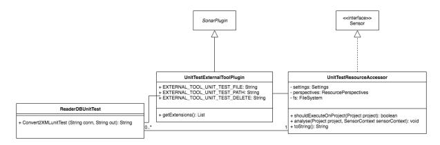
Figure 10: Class diagram of the unit test module/plugin
