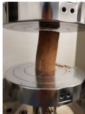
Figure 2. Cylindrical specimen deformed when unmolding by sample plasticity.
