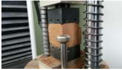
Figure 3. A cubic specimen in a compressive strength test.
