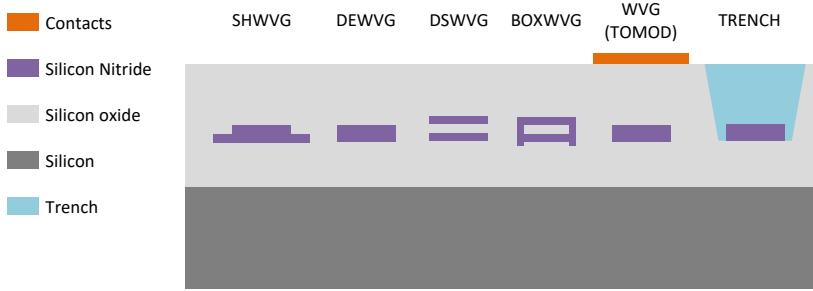
Figure 2.1: Silicon Nitride photonics platform cross-sections.
