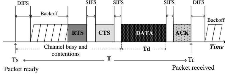
**Fig. 2** Transmission of a single packet in IEEE 802.11 DCF MAC protocol
