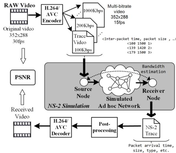
**Fig. 7** Simulation methodology: multi bit-rate video technique using H.264/AVC
