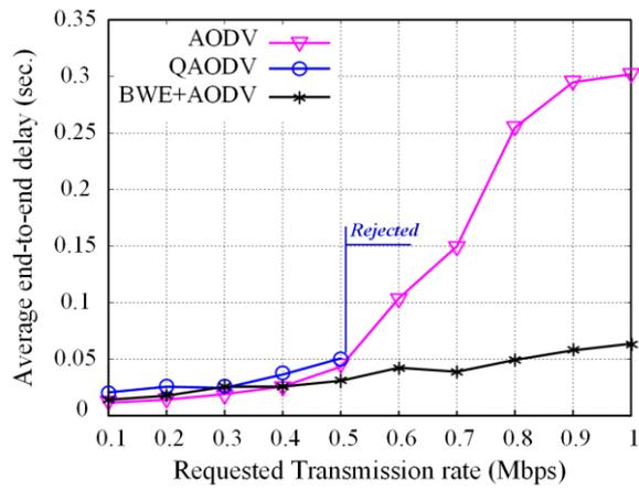
**Fig. 14** Average end-to-end delay with variable requested rate
