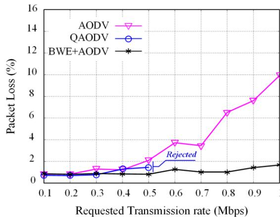
Fig. 13 Packet Loss with variable requested rate
