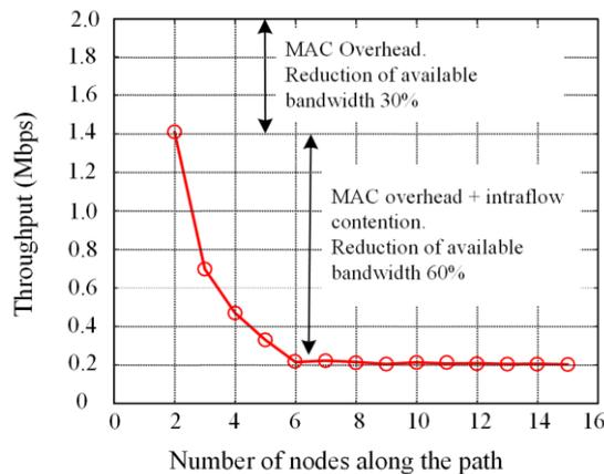
Fig. 1 Wireless link capacity as a function of the number of nodes along a route
