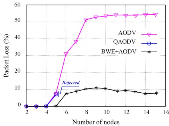
**Fig. 10** Packet Loss as a function of the route length
