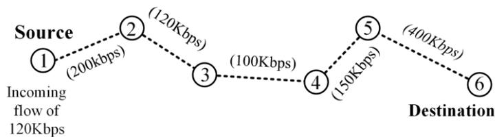
**Fig. 5** Example of wireless ad hoc network with the available bandwidth of each link
