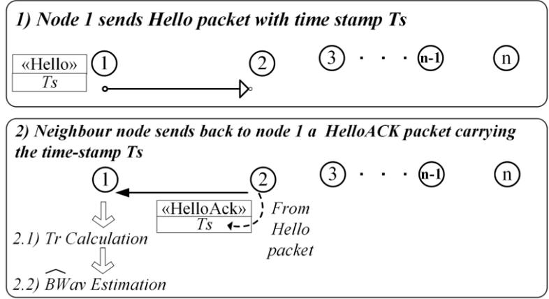
**Fig. 3** Bandwidth estimation using the Hello packets
