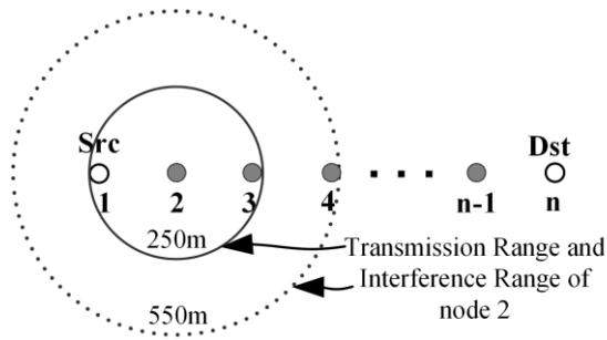
**Fig. 8** First scenario: static linear topology with variable length. The transmission and interference range for node 2 are shown
