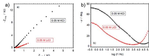
Fig. 7 (a) Nyquist and (b) Bode plots for electrochemical impedance spectroscopy of films of 3D G-SA prepared by pyrolysis at 900 °C on glassy carbon electrodes at air-saturated 0.05 M KCl and 0.05 M LiCl aqueous solutions. Bias potential of  $-0.65$  V vs. Ag/AgCl.
