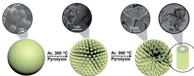
Scheme 2 Illustration of the hierarchical structure and morphological changes undergone by CTAC-SA with temperature.
