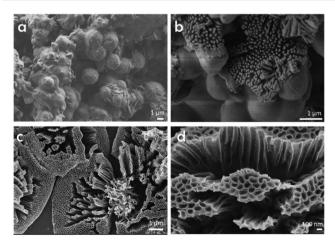
Fig. 3 SEM images of as-prepared CTAC–SA (a) and that treated at 300 (b) or 900  $^{\circ}$ C (c and d). Images (c) and (d) correspond, therefore, to the 3D G–SA sample referred in the text.
