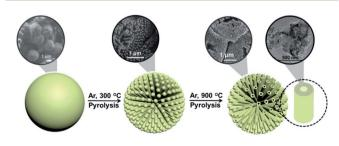
Scheme 2 Illustration of the hierarchical structure and morphological changes undergone by CTAC-SA with temperature.
