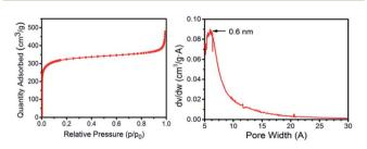
Fig. 2  $\,$  N\_2 adsorption isotherm at 77 K and pore size distribution measured by Ar for the 3D G–SA sample obtained by pyrolysis at 900  $^\circ C.$
