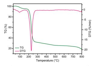
Fig. 4 TG profile and differential scanning calorimetry of the CTAC-SA sample
