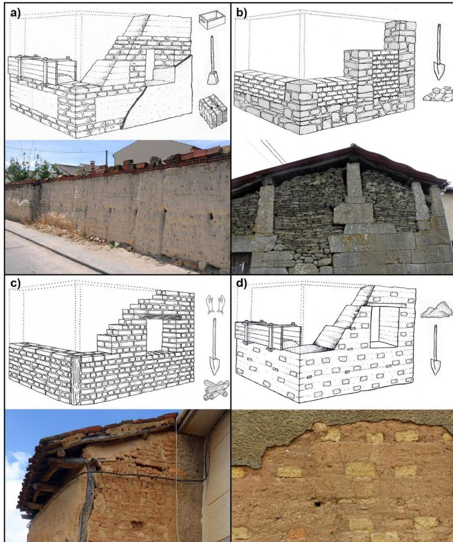
Figure 12. Other traditional walling techniques using earthen masonry (Drawings: SOStierra. Photos: Authors and E. Sevillano).
