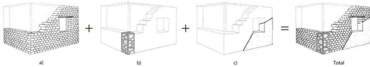
Figure 2. Different features of the cases considered in the constructive characterisation: a) Type of block and bond; b) External structural elements; c) Wall coating (SOSTierra).
