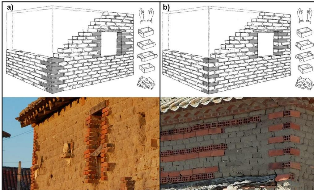
Figure 8. Adobe fabrics with insertions in corners (Drawings: SOSierra. Photos: Inventario de Arquitectura Vernácula de Extremadura and E. Sevillano).
