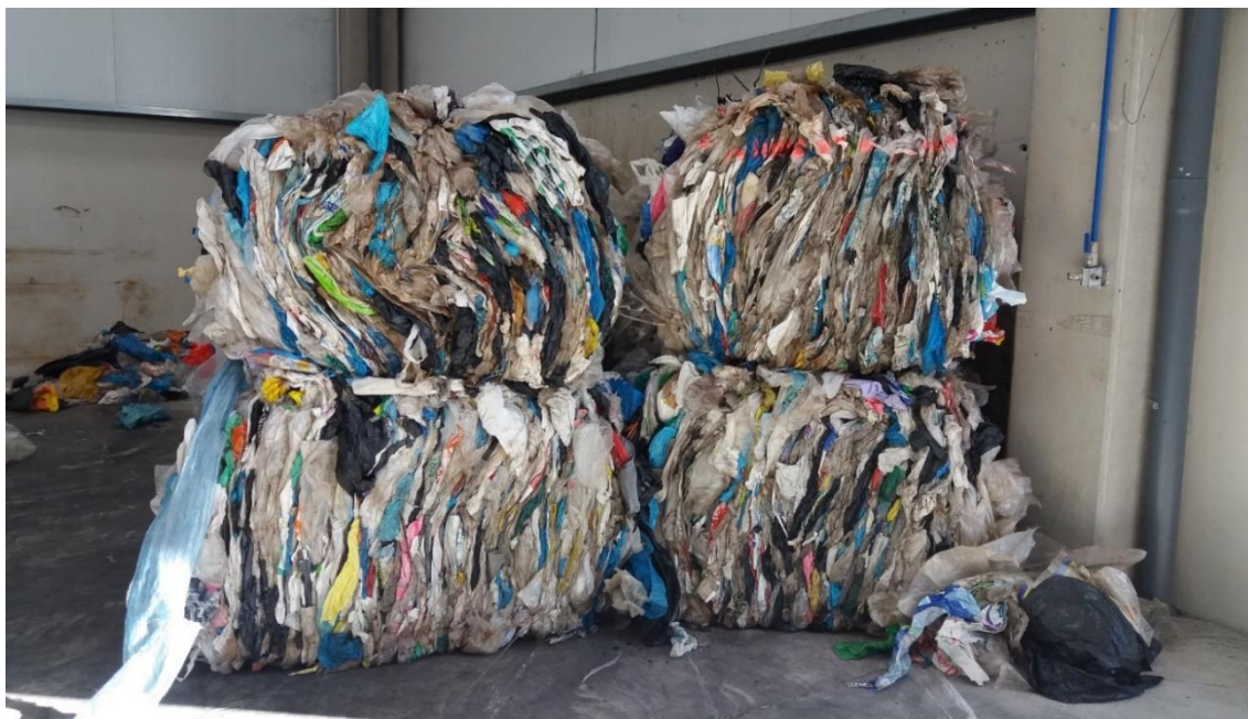
Supporting information – Figure 1. Colored plastic film waste bales recovered from mixed municipal solid waste at the Complex for Treatment of municipal Solid waste of Zaragoza (Urbaser facility).
