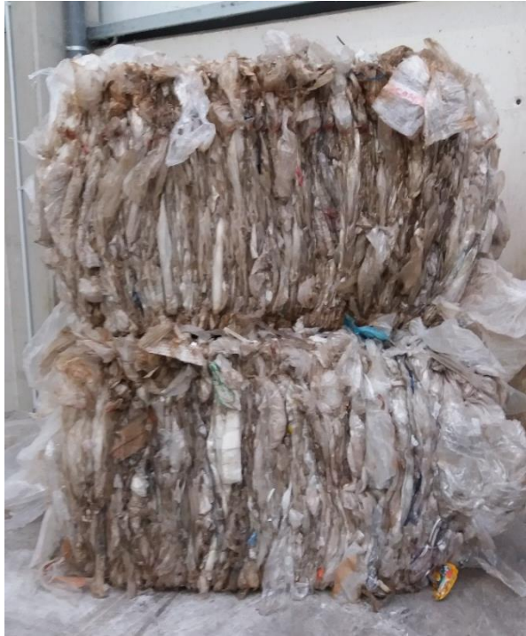
Supporting information – Figure 2. White plastic film waste bales recovered from mixed municipal solid waste at the Complex for Treatment of municipal Solid waste of Zaragoza (Urbaser facility).
