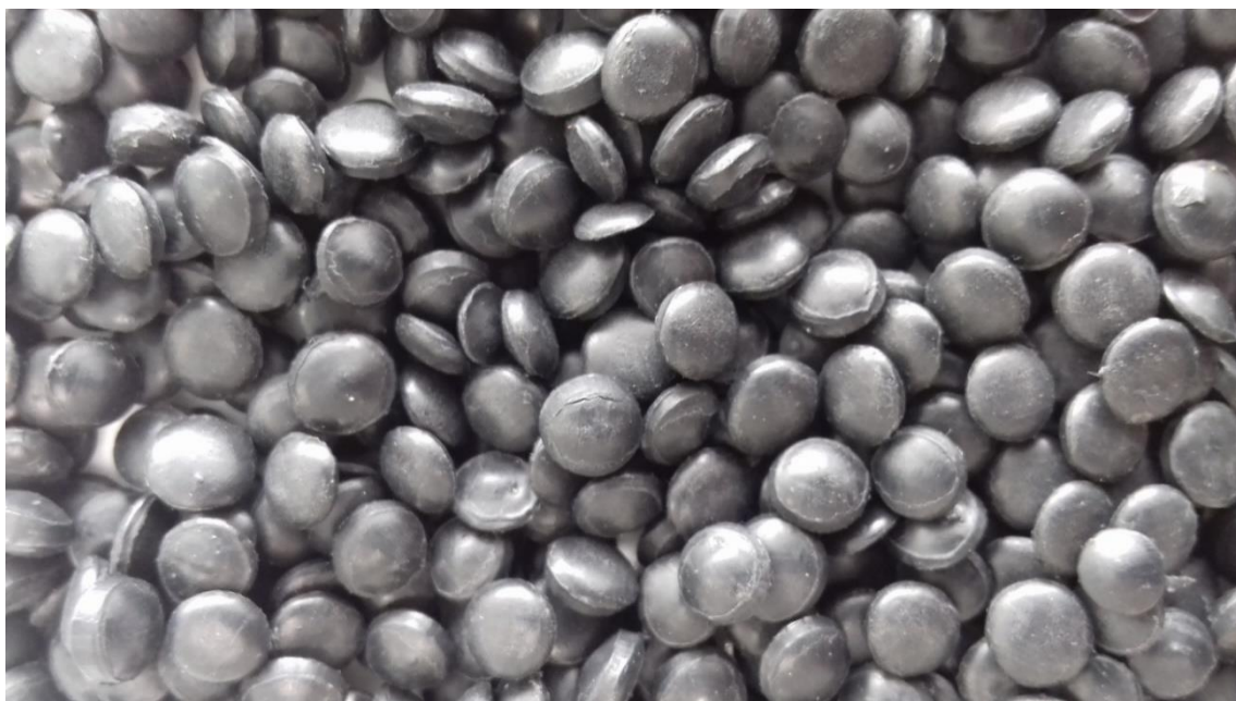
Supporting information – Figure 3. IPW: Industrial plastic waste provided by Granzaplast S.L. Plastics Recycling.
