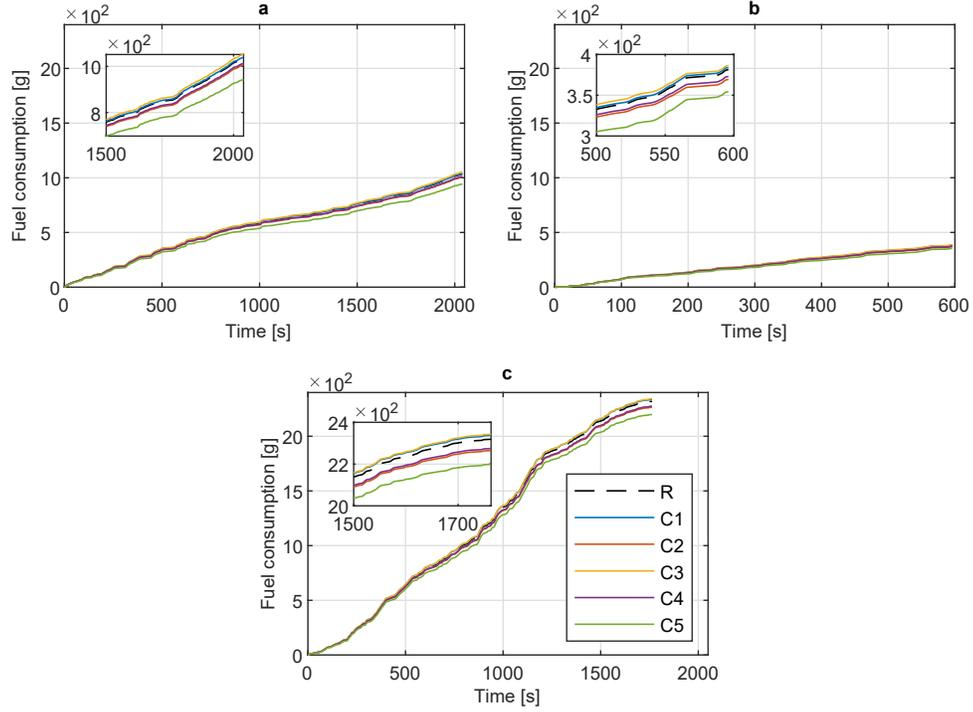
Figure 8: Accumulated fuel consumption for the urban cycle in Spain (a), urban cycle in UK (b) and rural cycle (c)
