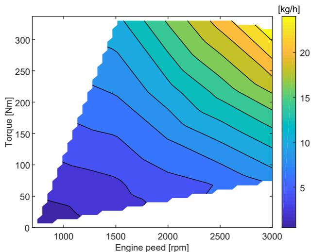
Figure 2: Fuel consumption map with reference oil used in the vehicle model
