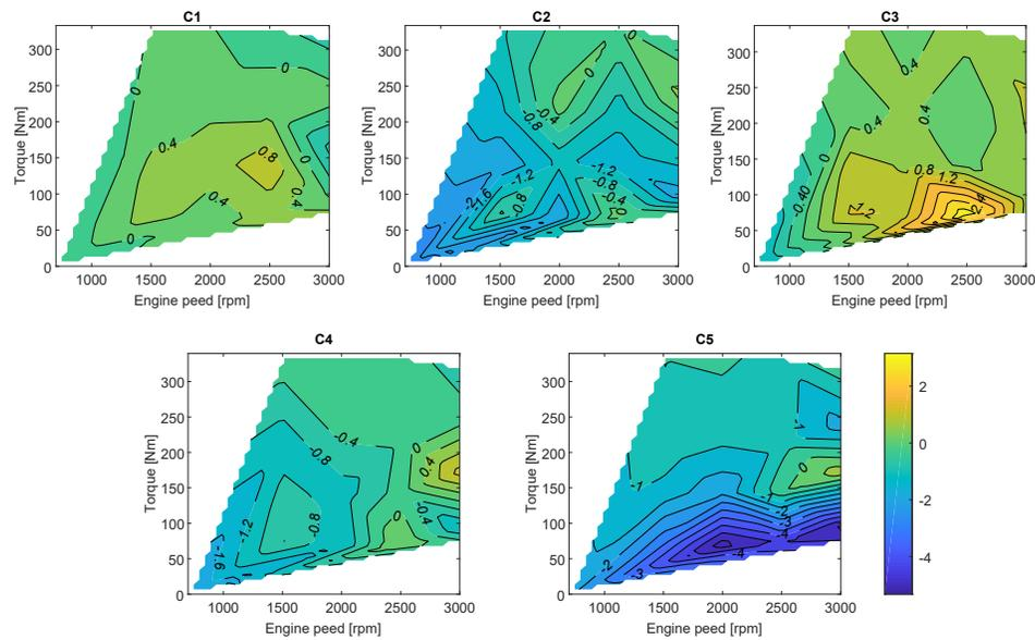
Figure 4: Fuel consumption differences between candidate and reference oils [%]
