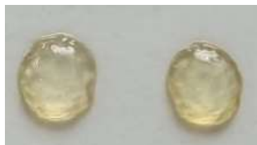
Figure 20. Example of oHA-Gel hydrogels (1:3 ratio) synthesized with bicarbonate buffer and Bloom 300 gelatin.
