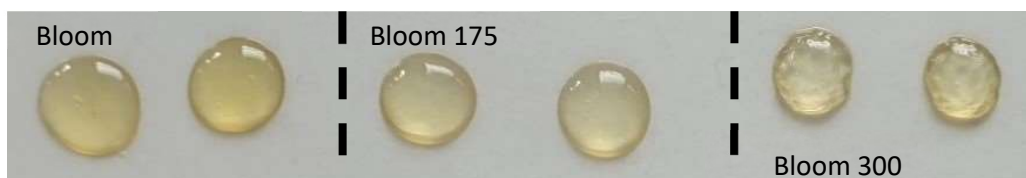
Figure 28. oHA-Gel hydrogels synthesized with bicarbonate buffer, ratio 1:3 (oHA-Gel) and made with different gelatin Bloom values (80, 175 and 300). Crosslinking time 1h at 37°C.
