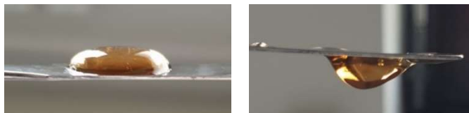
Figure 29. Representative image of oHA-Gel stable hydrogels after 7 days of soaking in F12 culture media with 1% of FBS in non-treated p24 non-treated well plates.
