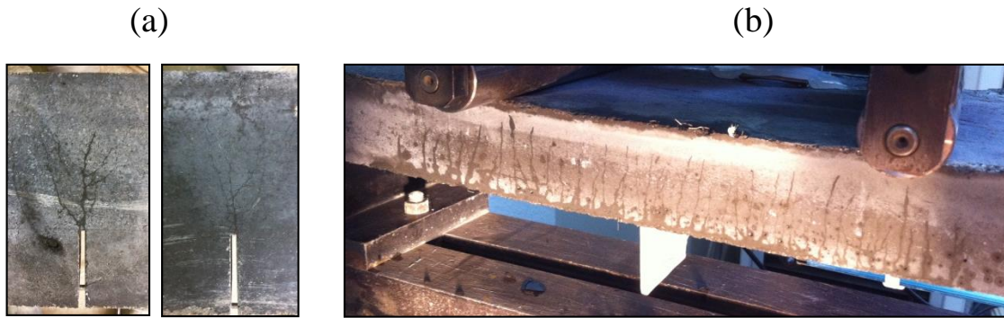
Figure 3. Micro-crack patterns in UHPFRC specimens: (a) regular specimens, and (b) slim specimens.
