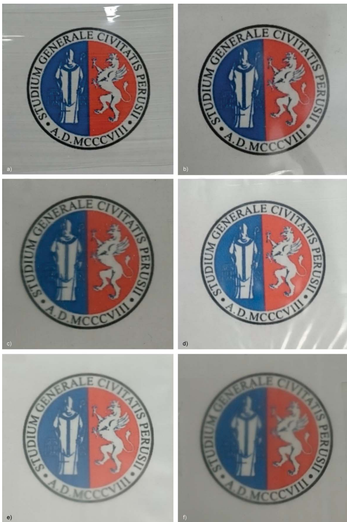
Figure 8. Visual appearance and contact transparency of films of: a) polyamide 1010 (PA1010); b) PA1010/polylactide (PLA); c) PA1010/PLA + epoxidized linseed oil (ELO); d) PA1010/PLA + epoxy-based styrene–acrylic oligomer (ESAO); f) polystyrene-glycidyl methacrylate random copolymer (PS-GMA).
