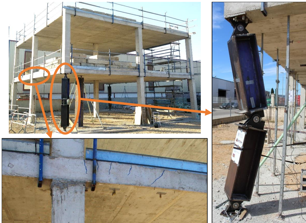
314 Fig. 16. Final state of the removed column and detail of cracking on P2 slab-column joint (1 st floor).
