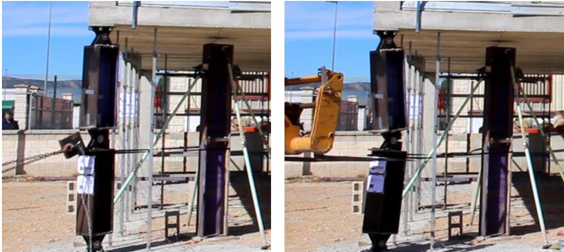
Fig. 6. Reproduction of the sudden failure of the column.
