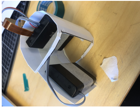
Figure 100: Battery placement on the hatch and inside.
