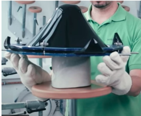
Figure 17: Lamination of inner hard socket - Start.
