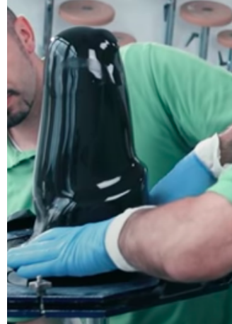
Figure 18: Lamination of inner hard socket - Finish.
