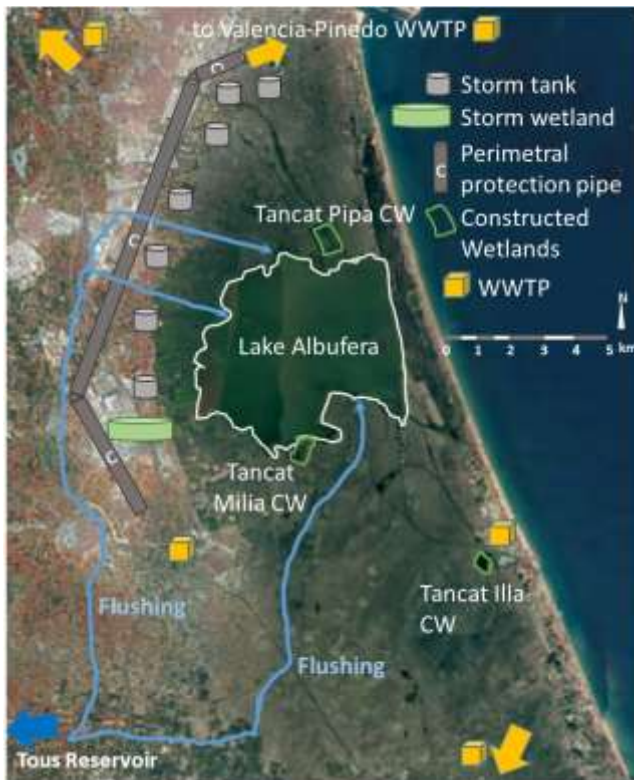
Fig.2. Restoring measures implemented in the Albufera of Valencia.
