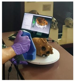
Figure 1: Data acquisition using the Artec Space Spider structured blue light scanner.
