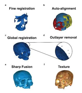
Figure 2: Workflow followed for processing the scan data in Artec Studio.
