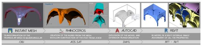
Figure 7: The GOG 10 workflow from mesh to parametric HBIM object.
