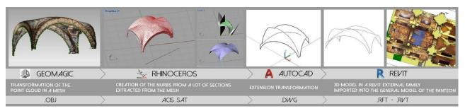
Figure 6: The GOG 9 workflow from mesh to HBIM object.
