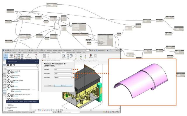
Figure 16: Isolation elements with specific "Activity ID" and two different constructive parameters.
