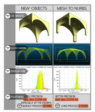
Figure 18: Comparison of the two different modelling methods.
