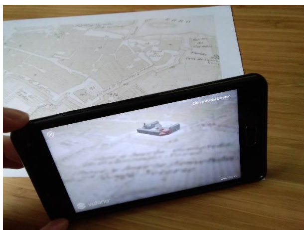
Figure 10: By means of the augmented reality, users can see the buildings over a printed plan in their mobile devices.
