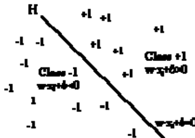
Figure 5. Linear classifier defined by the hyperplane H ( w \cdot x + b = 0 ).
