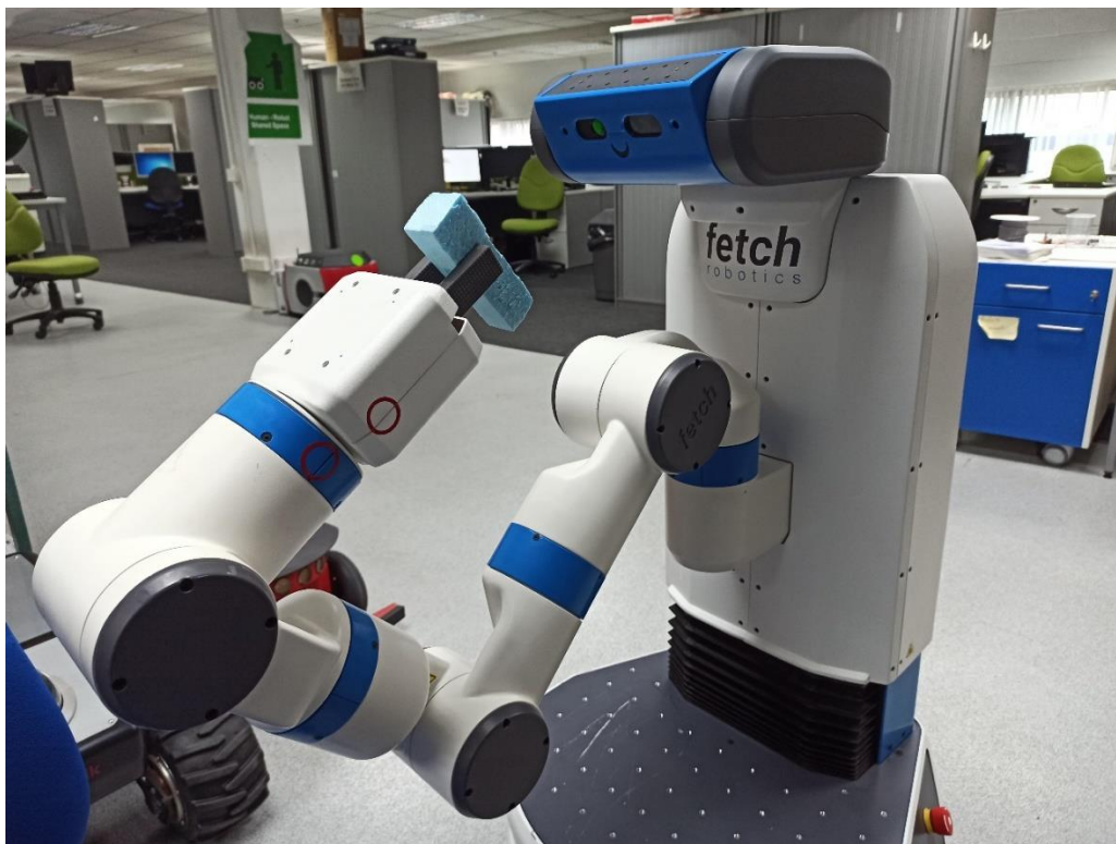
Figure 30. Fetch Robot with the prism picked up
