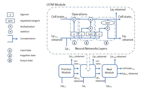
**Figure 1.** General scheme of an Long Short-Term Memory neural networks (LSTM) for  $L_p$ . The interaction between LSTM modules can be observed, as well as the three types of gates that make up an LSTM module.
