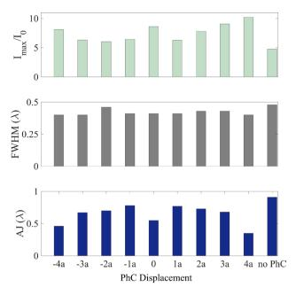
Figure 3. Acoustic parameter comparative for different PhC displacements inside the ABS cylinder.
