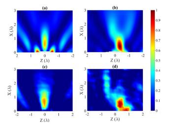
**Figure 5.** Normalized intensity planes ( $I/I_{max}$ ) for  $R = 4\lambda$  ABS cylinders. (**a**,**b**) correspond to numerical solutions with and without embedded 9 × 9 PhC rotated  $\theta = 15^{\circ}$ , respectively. (**c**,**d**) correspond to experimental measurements for same cases stated before.
