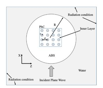
Figure 6. Scheme of the geometry and boundary conditions of the implemented FEM model.
