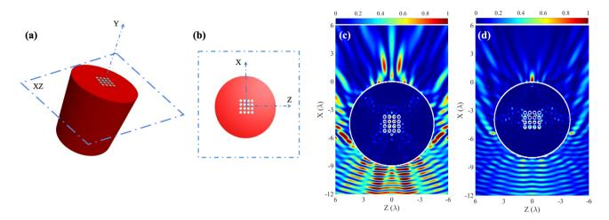
**Figure 2.** Schematic representation of the cylinder with a PhC embedded: (a) 3D view and (b) 2D view. Normalized intensity plane for numerical results for: (c)  $4.5\lambda$  radius ABS cylinder with an embedded  $4 \times 4$  PhC and (d)  $4\lambda$  ABS cylinder with an embedded  $4 \times 4$  PhC.
