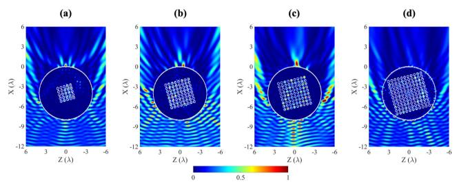
**Figure 4.** Normalized intensity plane  $(I/I_{max})$  for ABS cylinder with an embedded (**a**) 5 × 5, (**b**) 8 × 8, (**c**) 9 × 9 and (**d**) 11 × 11 PhC which is rotated  $\theta = 15^{\circ}$ .
