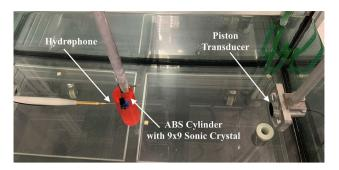
Figure 7. Photography with the detail of the different parts of the experimental set-up.
