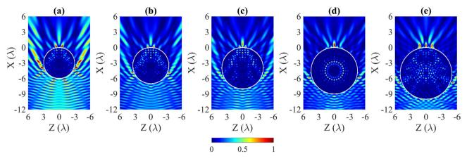
**Figure 1.** Normalized acoustic intensity planes ( $I/I_{max}$ ) for different ABS cylinder sizes of (**a**)  $3\lambda$ , (**b**)  $3.5\lambda$ , (**c**)  $4\lambda$ , (**d**)  $4.5\lambda$  and (**e**)  $5\lambda$ .
