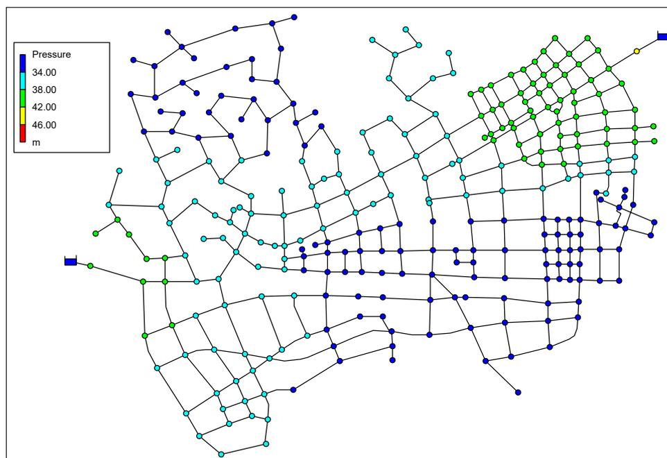
Figure 4. Topology and nodal mean pressure of JYN network.
