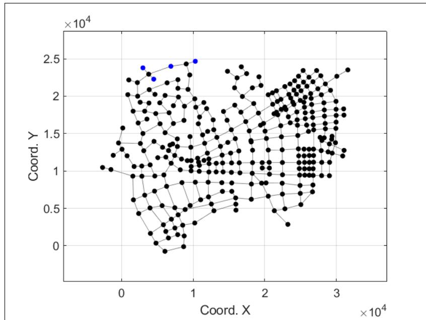
**Figure 7.** Layout of a sensor network with four sensors using only the sensitivity as input for Fuzzy DEMATEL.
