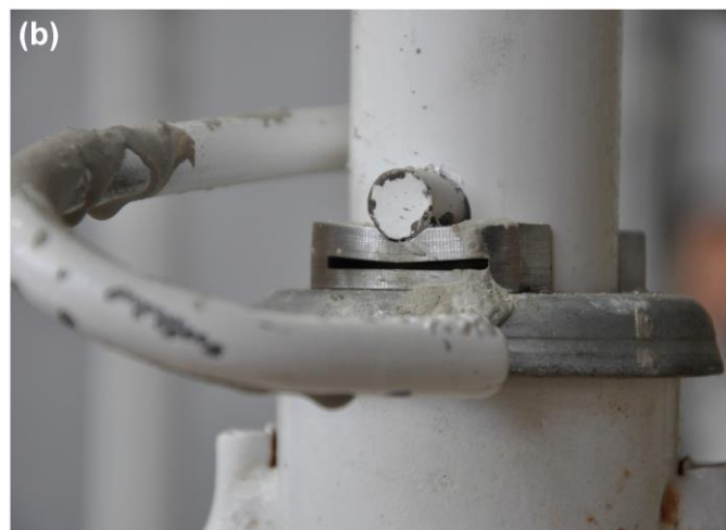
269 Fig. 8. (a) Force-displacement curve (shore 43-IL); (b) state of the LL at the moment of the maximum load of 270 17.7kN.
