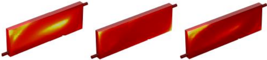
Figure 3.4 Qualitative fluid temperatura distribution adjacent to the active plate for the single flow box of figure 2 with L=24.2 cm, when qA=200 W and v_i=0.662 m/s (Base case). Left: water, Center: sunflower oil, Right: milk.
