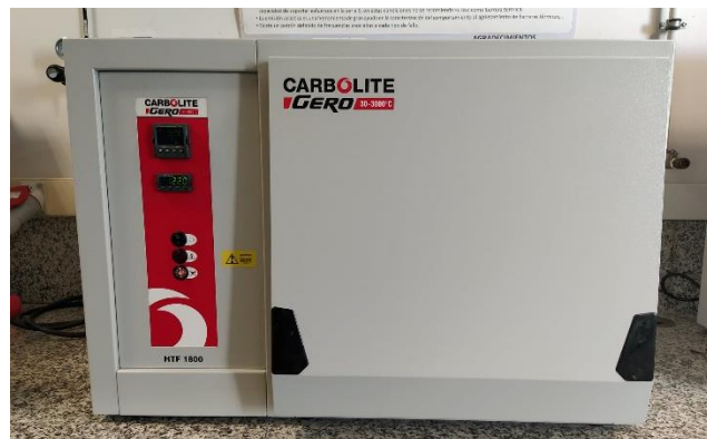
FIGURE 3-2. FURNACE USED FOR CONVENTIONAL SINTERING.
