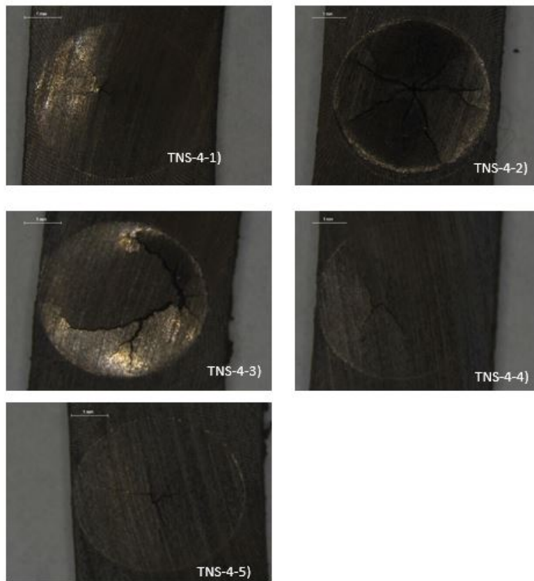
Figure 28: Image of the TNS-4 probes after the SPT
