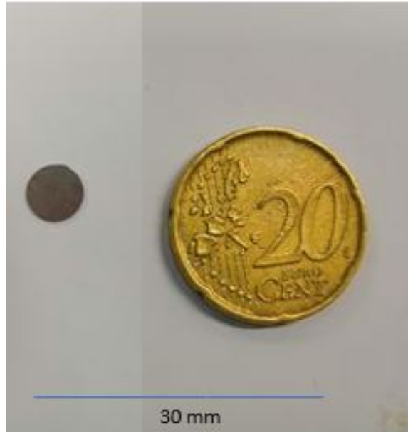
Figure 10: Image of a CPTi probe of SPT in comparison with a piece of 20cts
