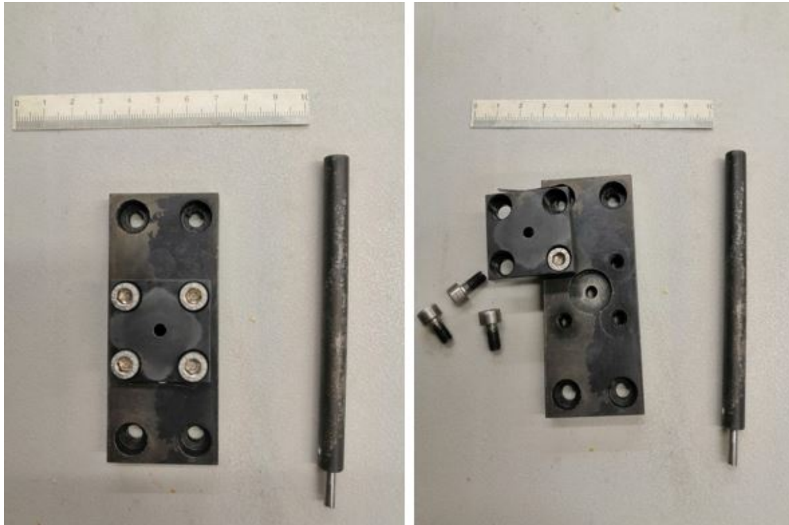
Figure 23: Image of the SPT device used for the test. The scale is in cm.
