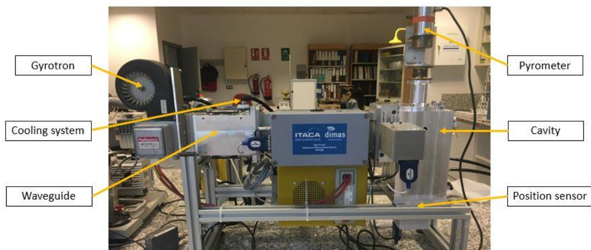
Figure 15: Annotated picture of the electrical single mode microwave.
