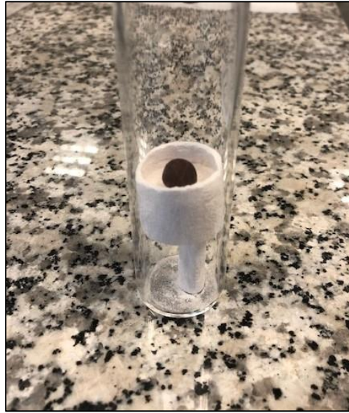
Figure 19: Disposition of a sample and its support in a quartz tube.
