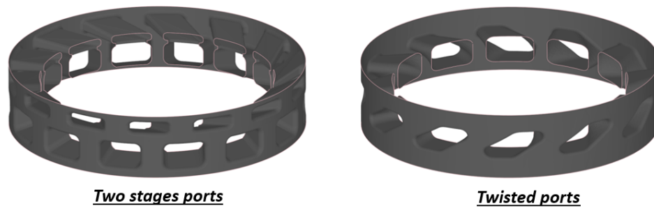
Figure 5.8. Two propositions of complex intake ports designs: two-stage ports (left) or twisted ports (right).
