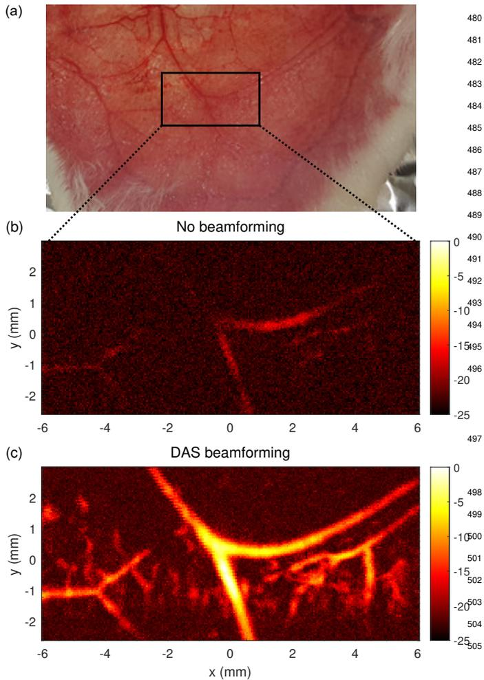
Figure 6: Ex vivo rabbit ear 2D PAM imaging. (a) Photograph of the excised rabbit ear, where the black rectangle indicates the scanned area. PAM images of the rabbit ear vasculature comparing (b) no-beamforming and (c) dynamic beamforming.
