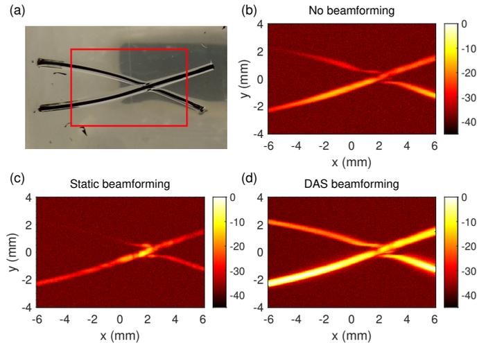
Figure 4: **2D photoacoustic images using gelatin phantoms.** (a) Photograph of the surface of the phantom including polyethylene tubes at its surface. The red rectangle represents the scanned area. 2D photoacoustic images of the gelatin phantoms using a single set of experimental data, applying (b) no-beamforming, (c) static beamforming aimed at the crossing point of the PE tubes and (d) dynamic beamforming aiming the focusing point at the focal spot of the laser for every scanned point.
