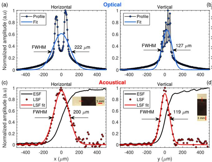
Figure 3: **Lateral resolution evaluation.** (a) Horizontal and (b) vertical optical  $x$ - $y$  experimental profiles of the laser beam at its focus and beam spot size from Gaussian fitting at FWHM. (c) Horizontal and (d) vertical ESFs, LSFs and corresponding Gaussian fittings obtained from photoacoustic measurements.
