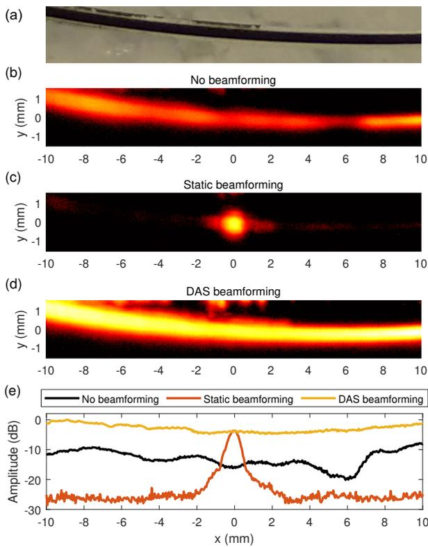
Figure 5: SNR comparison between beamforming strategies. (a) Photograph444
