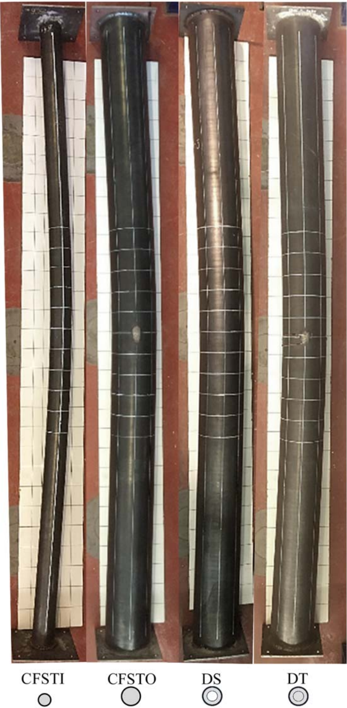
Fig. 5. Columns after test.
