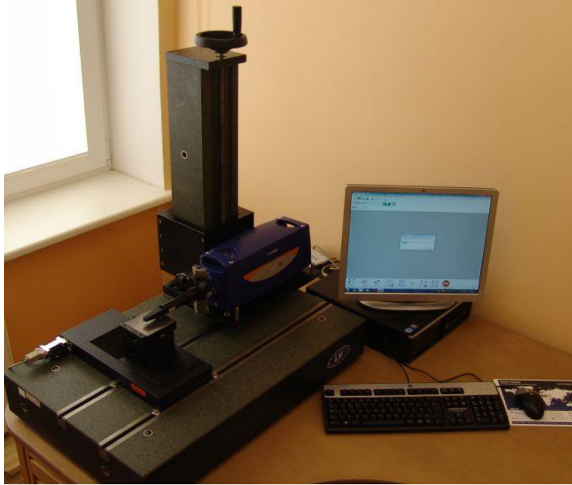
Fig. 5.2. 3D surface topography measurements with Talysurf Intra 50 contact measuring device
