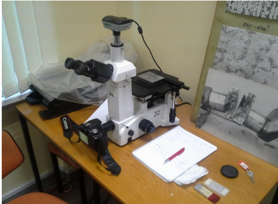
Fig. 5.4. Microscope used to take the surface topography photos
