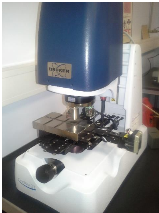
FIG. 5.3. 3D surface topography measurements on the Bruker Contour 3D optical measuring device
