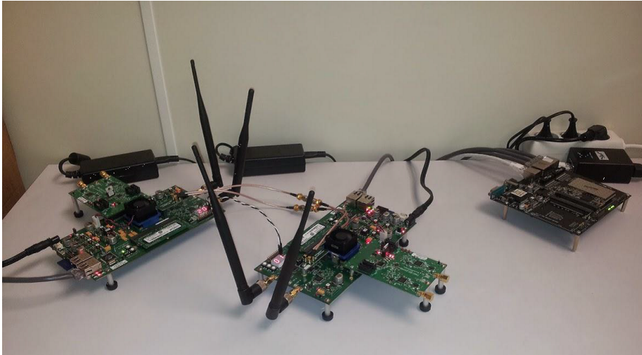
Figure 3.2: SDR scheme used for waveform implementation
