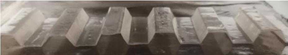
A row of seven white, rectangular test specimens with a central notch, arranged on a dark surface. The specimens show increased translucency.                                                       |
