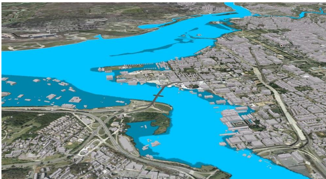
Figure 16. Flood event and buildings in the floodway. This can be used to determine which parcels fall inside the flood event, to determine potential costs of damage.
