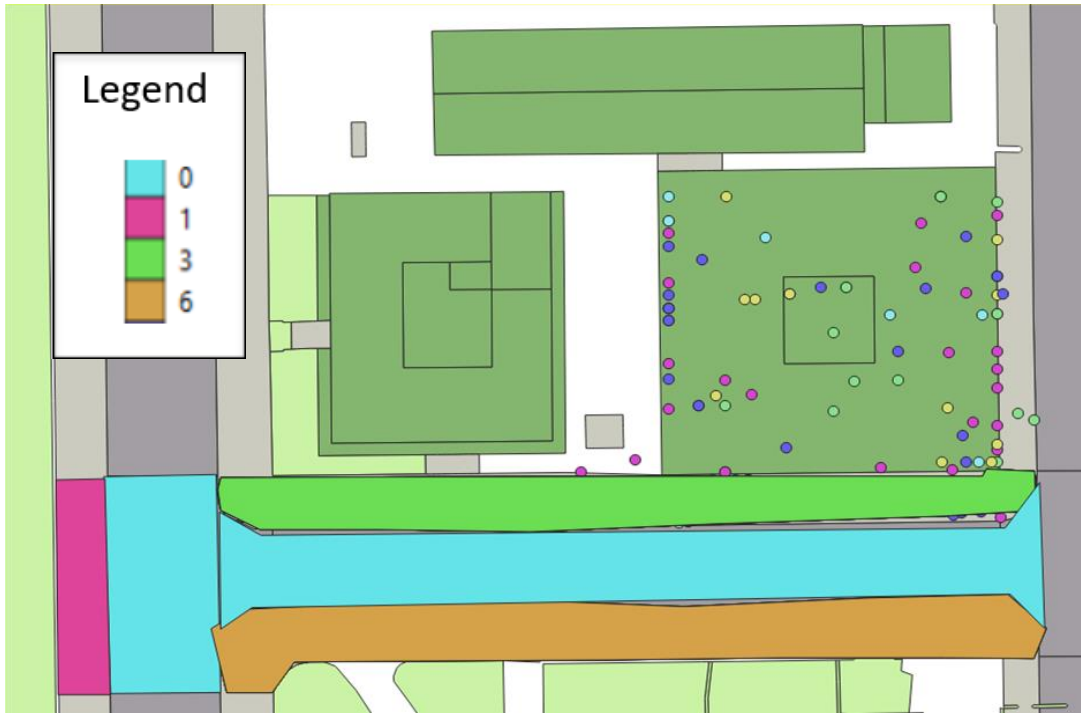
Figure 91. Different surfaces coloured depending on how many defects there are.
