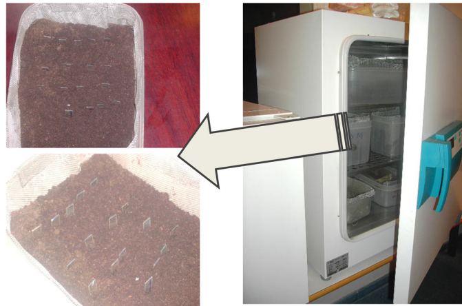
Figure 3-2 Soil burial test in a culture oven at 28 °C.
