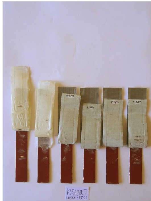
Figure 5.5.18. Specimens faced with RTS of K(3)A(4)E and stored at 80 % RH after the RTS (white strips) were peeled apart from the paint-mock-ups (red strips).
