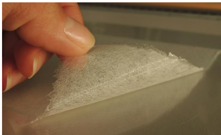
Figure 3.1.1. Remoistenable temporary support after the application and the drying of the adhesive.
