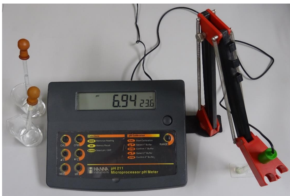
Figure 4.2.4. Measurement of the pH of dried adhesive dispersion by a specific electrode for measurement of surfaces.
