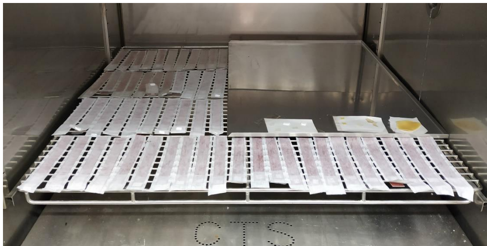
Figure 5.5.4. Specimens stored in the climate chamber at 23 \pm 1 °C and 80 \pm 5 % RH for a minimum of 72 h.
