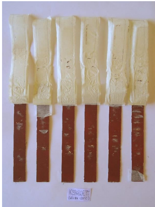
Figure 5.5.12. Specimens faced with RTS of K(3)A(4)E and stored at 45 % RH after the RTS (white strips) were peeled apart from the paint-mock-ups (red strips).
