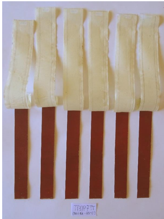
Fig. 5.5.14. Specimens faced with RTS of T(3)P7 and stored at 80 % RH after the RTS (white strips) were peeled apart from the paint-mock-ups (red strips).
