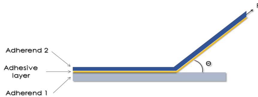
Figure 5.5.1. Schematic representation of generic peel test.
