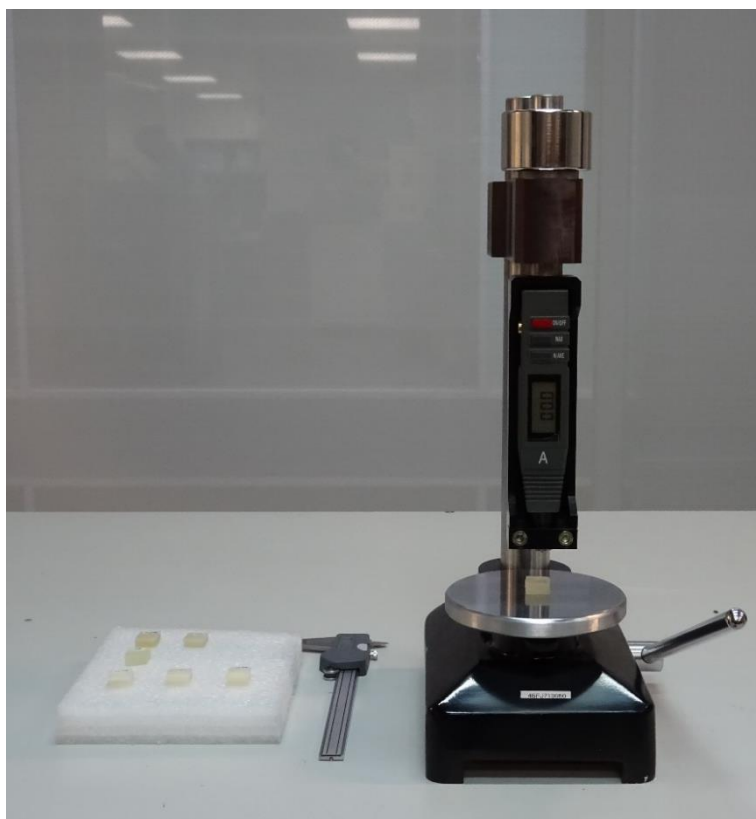
Figure 4.2.2. Hardness test. Measurement of samples of minimum thickness of 6 mm.
