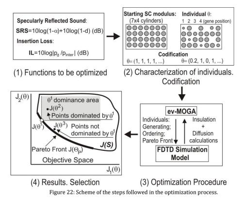
An outline of the optimization procedure is shown in Fig. 22. First (step 1), it is necessary to define the functions to be optimized, generally referred to as optimization objectives or cost functions. In our case, we want to design devices with high levels of
