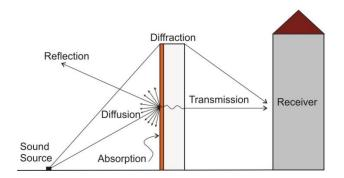
Figure 1: Diagram of the acoustic performance of a screen
