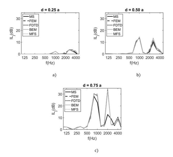
Figure. 29. *IL* vs frequency, in one-third octave bands, for all the considered methods: a) d = 0.25 a; b) d = 0.5 a; c) d = 0.75 a.
