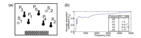
Figure 14: (a) Scheme of arrangement of the instrumental used (two sources and five microphones) in the test given by EN 1793-1:1997 norm.; (b) Variation of αS as a function of the frequency.
