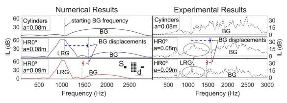
Figure 20: Numerical (continuous line) vs experimental (dashed line) IL results for three PC cases: Cylinders with a=0.08 m, HR0° with  $a\frac{1}{4}0.08$  m, and HR0° with a=0.09 m. An outline of the experimental setup is shown at the bottom left.
