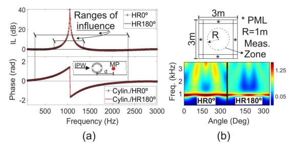
Figure 18: Analysis of the influence of the three possible mechanisms responsible for interference in the case of single scatterers; (a) absorption spectra (upper part) and phase shift spectra (lower part) for HR0° and HR180°. In the inset, you can see a schematic of the numerical model used; (b) an outline of the anechoic model used to simulate the directivity of both HR (upper part); the directivity results can be seen at the bottom.
