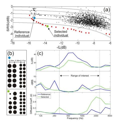
Figure. 25. Optimization results for the bi-crystal case. (a) Objective space where the initial population, the Pareto Front and both the selected and the reference individuals are remarked; (b) Devices considered, the selected individual and the reference one (c) Acoustic performance of both individuals, reference (blue continuous line) and selected (green dashed line). IL, -SRS and d spectra are shown in the frequency range targeted.
