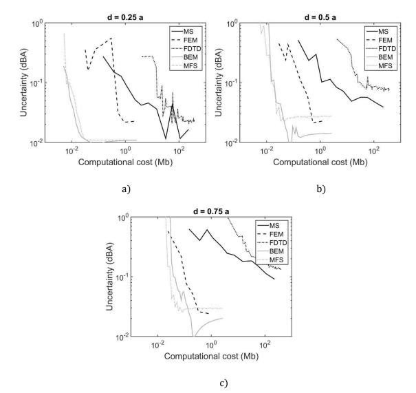
Figure. 30. Uncertainty of IL<sub>A,tr</sub> versus computational cost for all the studied methods: a) d = 0.25 a; b) d = 0.5 a; c) d = 0.75 a.
