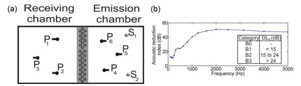
Figure 15: (a) Scheme of arrangement of the experimental set up used (two sources and five microphones) in the test given by EN 1793-2:1997; (b) Experimental values of the index R.
