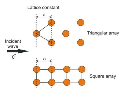
Figure 8. Bidimensional sonic crystals, triangular and square.
