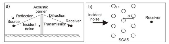
Figure 12: (a) Scheme of a classical acoustic barrier; (b) Plan view of a Sonic Crystal Acoustic Screen.
