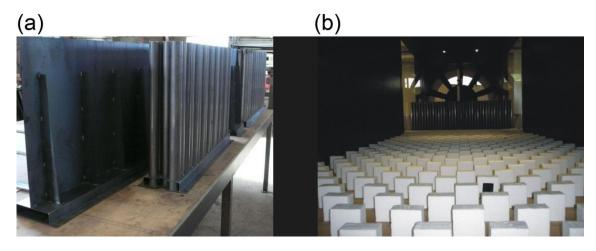
Figure 16. (a) Partial view of the scale model of both classical AB and SCAS; (b) View of the arrangement of obstacles inside the wind tunnel
