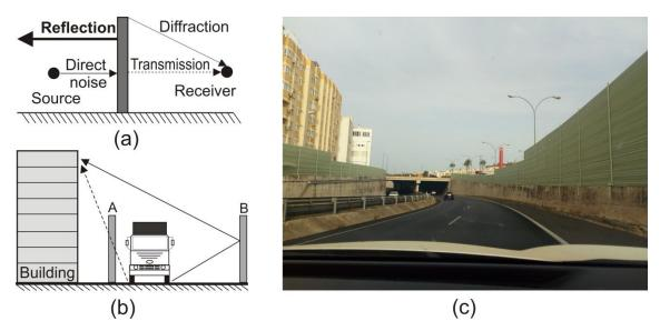
Figure 21: (a) Scheme of the acoustic performance of AB; (b) Scheme of the problems created by the specularly reflected noise; (c) A picture taken at one of the entrances to the city of Cádiz (Spain) to illustrate the described situation.
