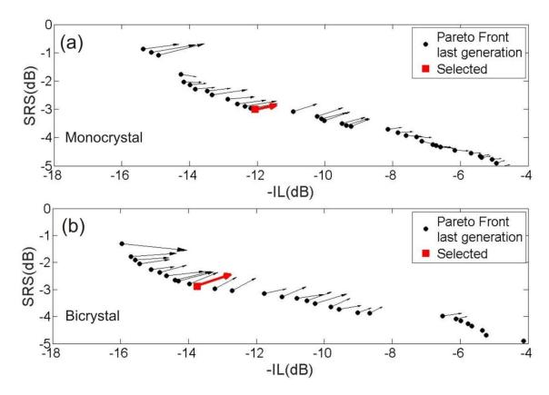
Figure. 26. Pareto front with the robustness vectors of the radii for both cases analyzed. Both selected individuals are represented by a red square, and the particular robustness of both individuals is shown by a thick red vector. (a) mono-crystal; (b) bi-crystal.
