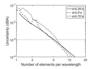
Figure. 28. Evolution of the uncertainty on  $IL_{A,tr}$  (in dB(A)) with increasing number of elements for the BEM.
