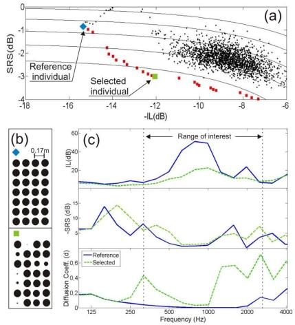
Figure. 24. Optimization results for the mono-crystal case. (a) Objective space where the initial population, the Pareto Front and the selected and the reference individuals are remarked; (b) Analyzed devices; (c) Acoustic performance of both individuals, reference (blue continuous line) and selected (green dashed line). IL, -SRS and d spectra are shown in the target frequency range.
