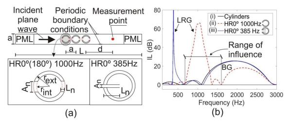
Figure 17: (a) Numerical 2D model to analyze the BG/LRG interactions. The typology of the scatterers is shown at the bottom; (b) IL spectra for the three considered arrays.
