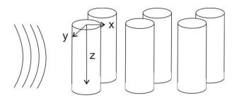
Figure 7:Bidimensional sonic crystal formed by cylindrical scatterers.
