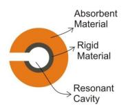
Figure 11. Multi-physics acoustic scatterer section
