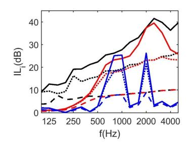
Figure. 34. Estimated insertion losss levels, *IL*<sub>i</sub> along the analyzed frequency range, for the 9 sound attenuation samples in one-third octave bands: different situations I, II, III represented, respectively, as continuous, dotted and dashed lines; on the other hand, traditional noise barrier, sonic crystal noise barrier with absorbent scatterers and classic sonic crystal noise barrier represented in lines black, red and blue, respectively.
