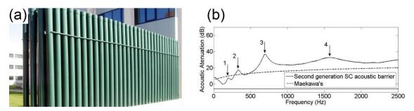
Figure 13: (a) Example of first generation SCAS; (b) Simulated attenuation spectrum of the SCAS.
