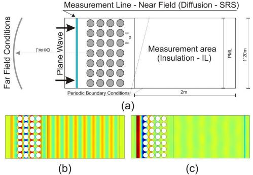
Figure. 23. (a) Scheme of the simulation model, based on FDTD, used to acoustically characterize the individuals generated by ev-MOGA; (b) and (c) Examples of acoustic pressure fields, in Pa, for frequencies outside (1370 Hz) and inside (1000 Hz) the bandgap respectively.
