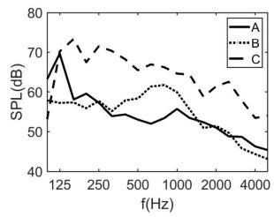
Figure. 33. Sound spectra in one-third octave frequency bands of the noise traffic recordings selected for the listening tests: (A) light vehicles at urban speed; (B) light vehicles on motorways; (C) motorcycles on motorways.
