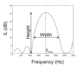
Figure 9 Insertion Loss (dB) vs frequency (Hz) of a SC.
