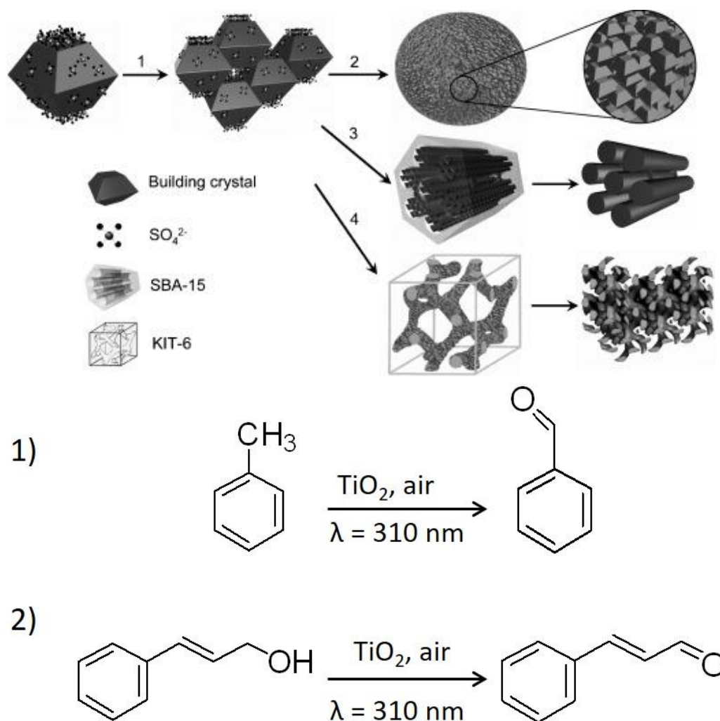
Figure 12. (Top) Synthesis of mesoporous single-crystal-like TiO 2 . 1) Formation TiO 2 crystal clusters with preferential exposure of the (001) planes from component crystals of which (001)
