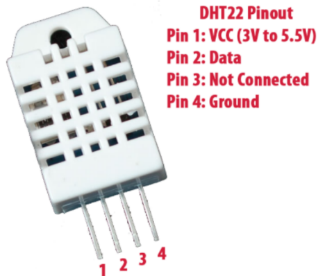
Figura 2.2: Sensor DHT22
