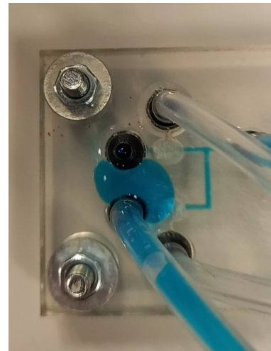
(f) Liquid routing with one valve under vacuum and the other valve under vacuum.
